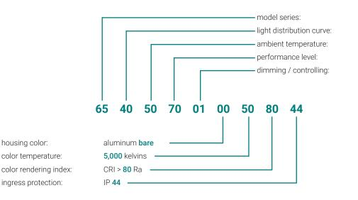
tempLED RayLine Eco V3 INTENSE [approx. 40° symmetric narrow beam] up to +50 degrees Celsius 70 watts and up to 13,650 lumens<sup>1</sup> DALI-2 dimming
