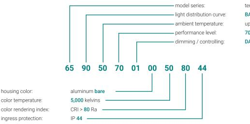
tempLED RayLine Eco V2 BATWING [approx. 90° symmetric wide beam] up to +50 degrees Celsius 70 watts & 11,900 lumens DALI-2 dimming
